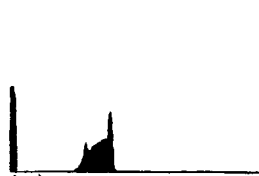
Fig. 3.—The initial and 1400-minute descending boundaries for hypoiodite oxidized hydrolyzed cotton cellulose; 0.5% concentration in 0.1 N cupriethylenediamine solution; current, 30 ma.; field strength, 3.01 v./cm.
